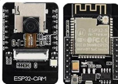
Gambar 1. ESP32 CAM
